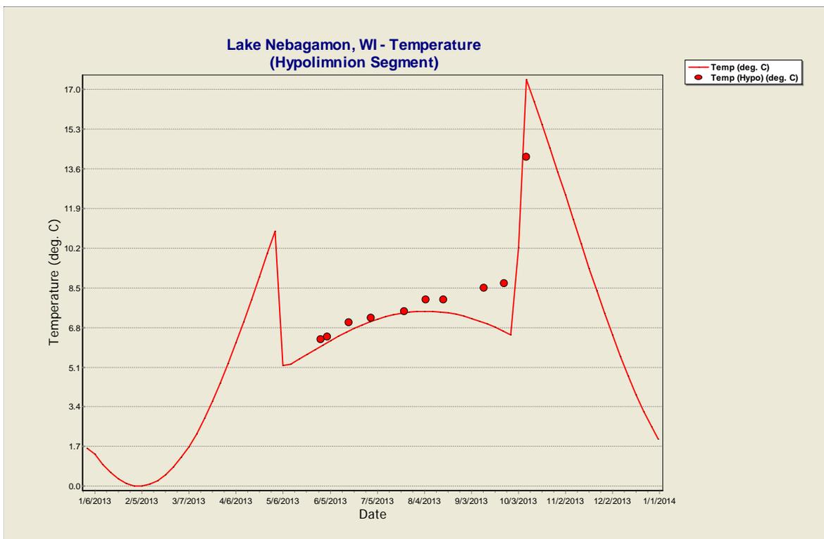
Figure 16.1 Validation of temperature representation in the AQUATOX model.
