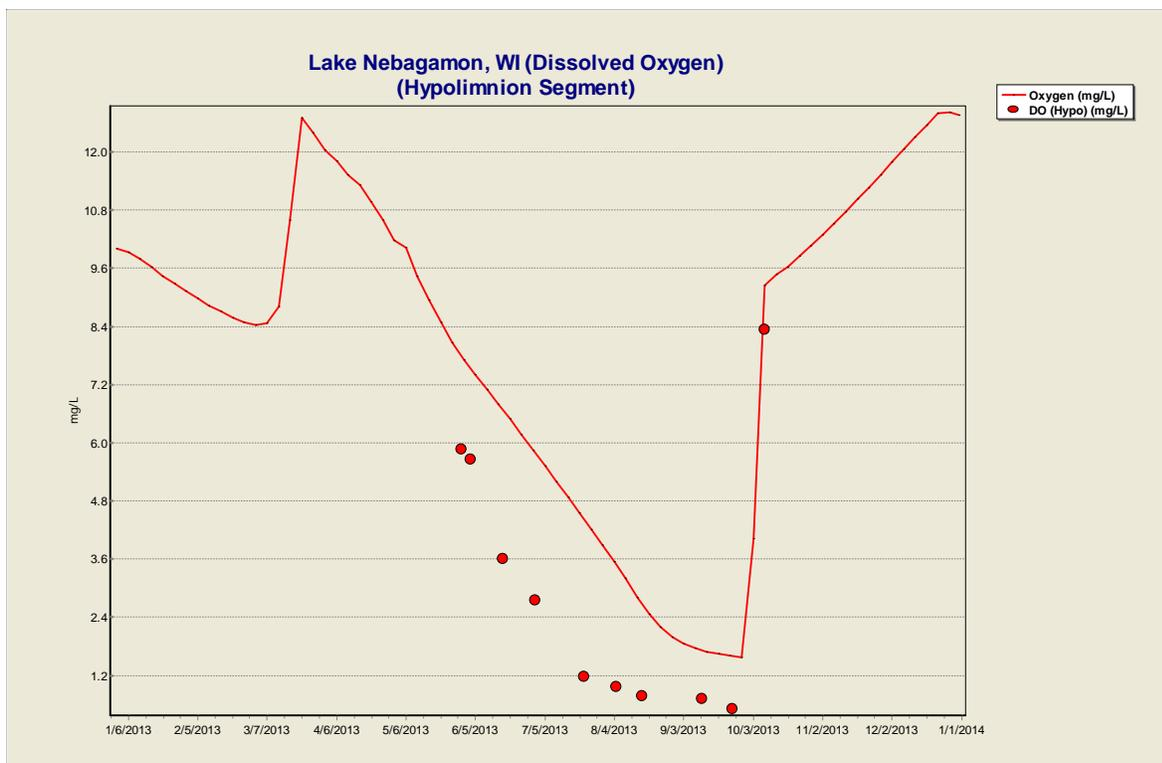
**Figure 16.2** Validation of dissolved oxygen representation in the AQUATOX model.
