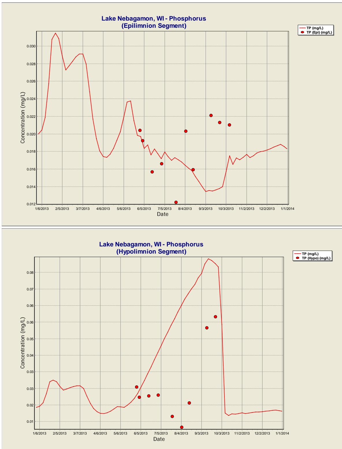
Figure 16.3 Validation of nutrient parameters in the AQUATOX model.
