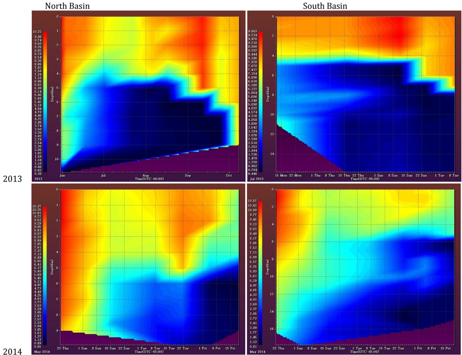
**Figure 11.3** Dissolved oxygen stratification in the north and south basins of Lake Nebagamon in 2013 and 2014.
