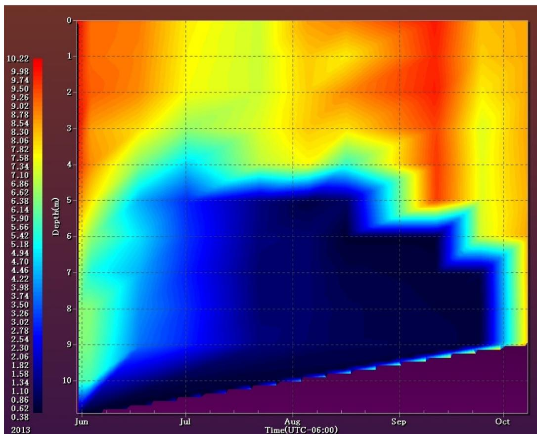
**Figure 5.11.** Vertical profiles of oxygen concentrations in Lake Nebagamon (north basin). Red colors indicate the areas of highest oxygen concentration.
