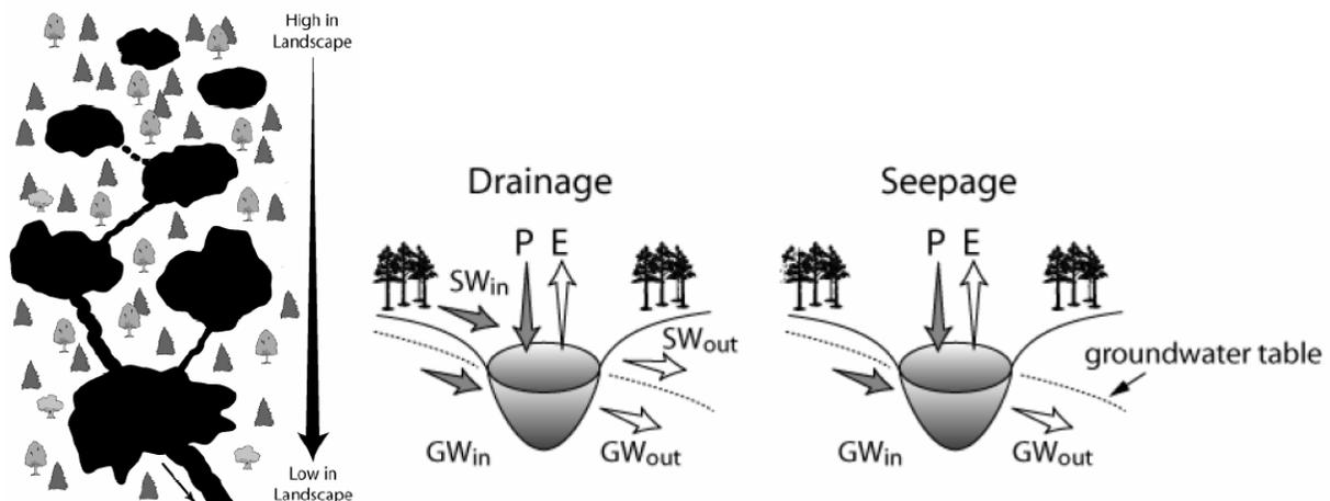
**Figure 5.6.** Conceptual diagram of “landscape position” and the differences in hydrologic processes between drainage and seepage lakes. Modified from Magnuson et al. 2006.
